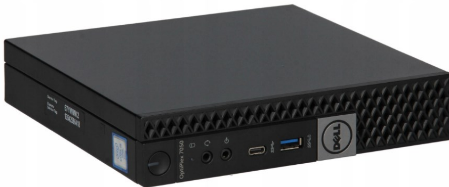
DELL OptiPlex Micro 7050 Intel Core i7-7700 @ 3.6 GHz, 32 GB RAM
