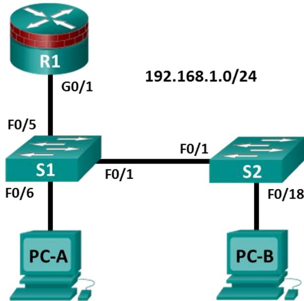
**Note:** ISR G1 devices use FastEthernet interfaces instead of GigabitEthernet interfaces.
