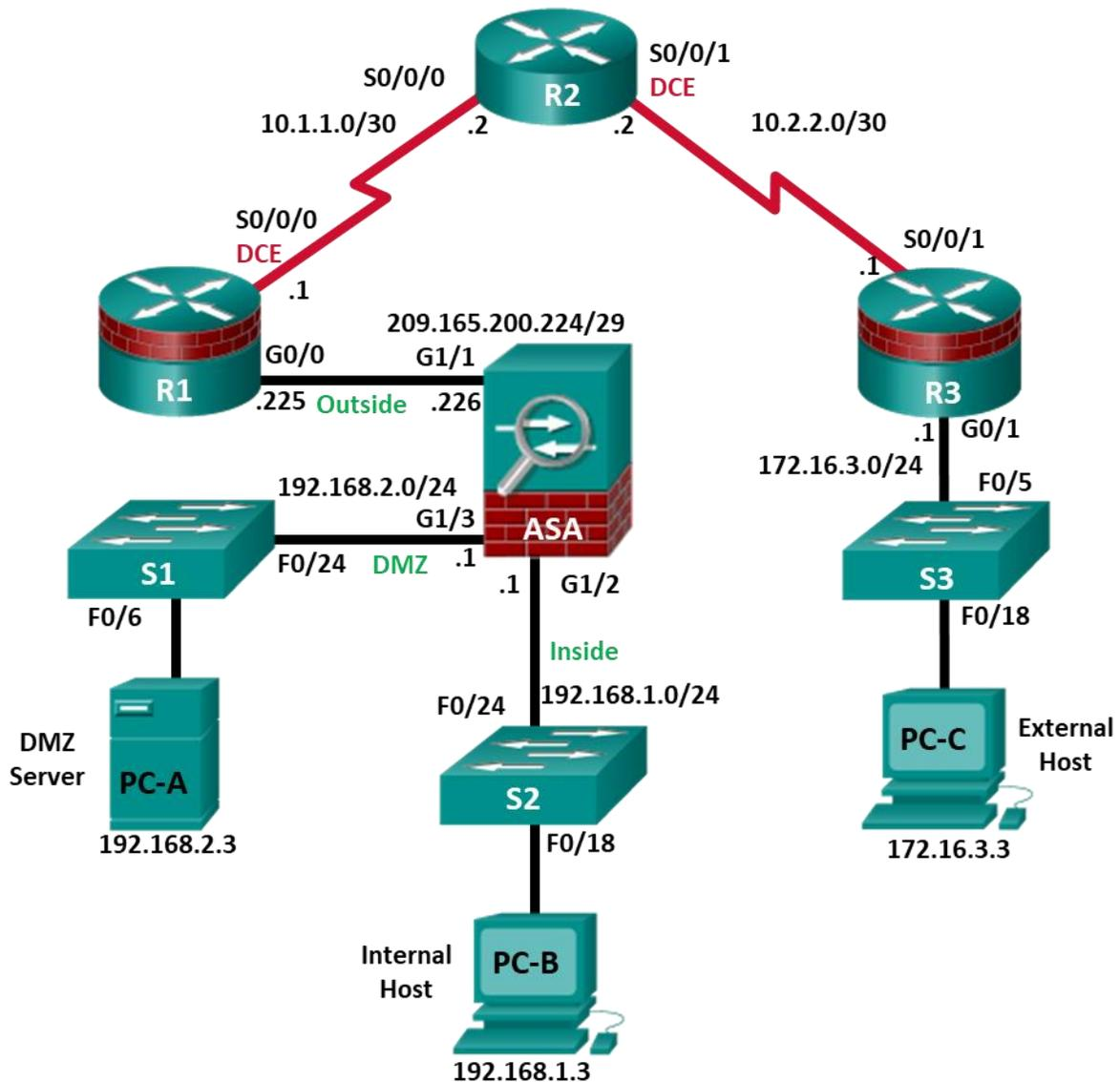
**Note:** ISR G1 devices use FastEthernet interfaces instead of GigabitEthernet interfaces.
